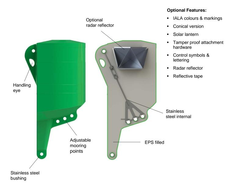
Note: actual radar reflector may differ from the radar reflector shown in the renderings.
